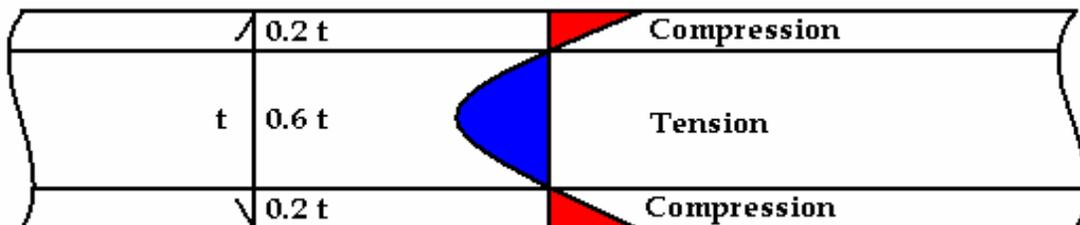
Conventional scoring uses the guidelines of 8-10% fissure depth or nearly  $0.1t$  whereas in pressure scoring the guideline is 17-20% fissure depth or nearly  $0.2t$ .
